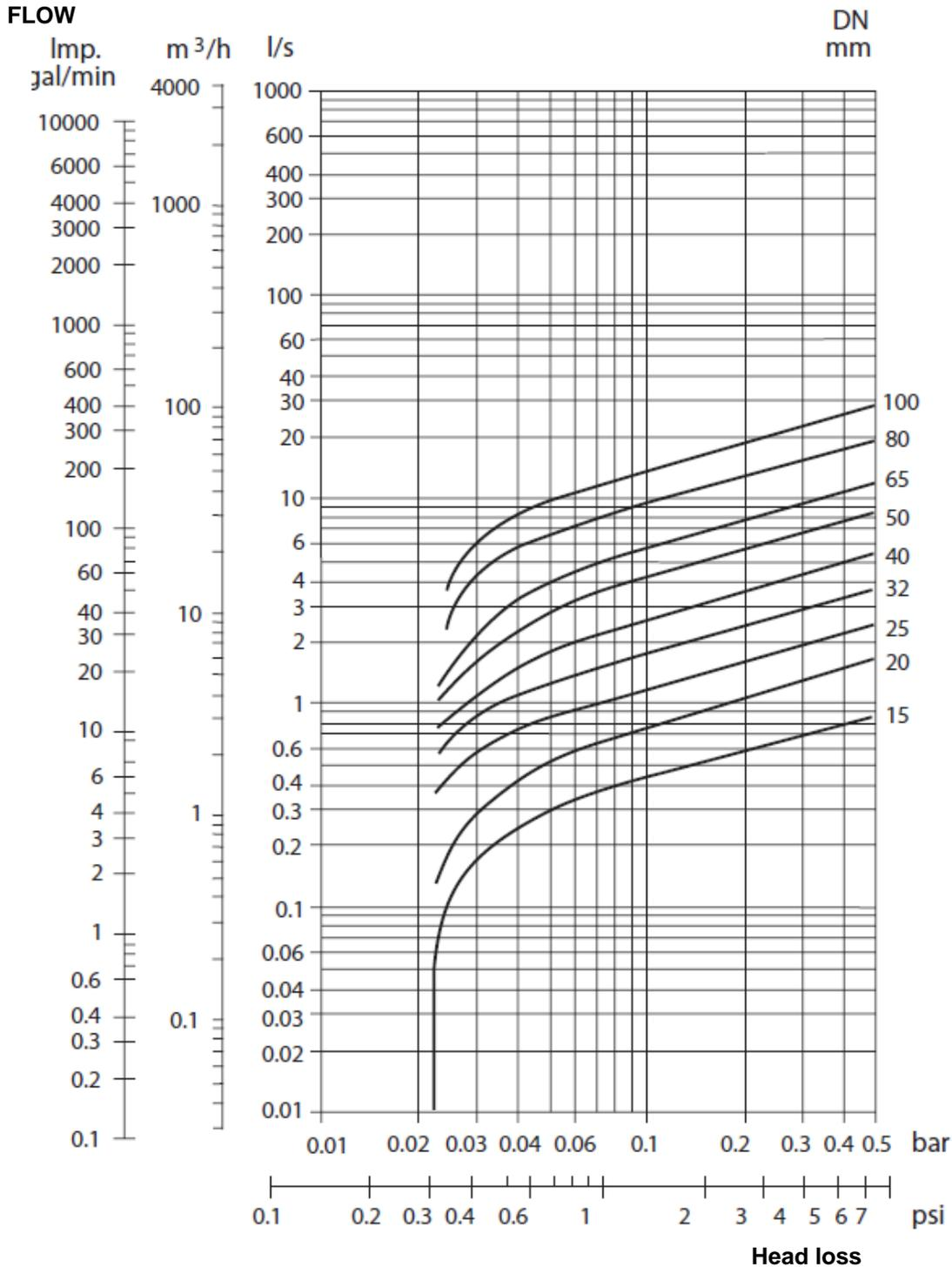
**BRASS WAFER SPRING CHECK VALVE PN16**
