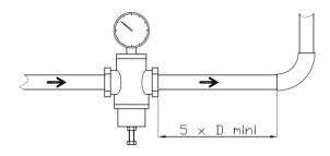
\_\_\_\_\_ Plan a stop valve upstream to the 684 HP. This one is not necessarily tight in zero flowrate and cannot be considered as an isolating valve.
