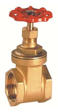
Size : DN 1/4" to 4" Ends : Female - Female BSP Min Temperature : -10°C Max Temperature : + 80°C Max Pressure : 16 Bars Specifications : Rotating non rising stem Inside screw stem Full bore
