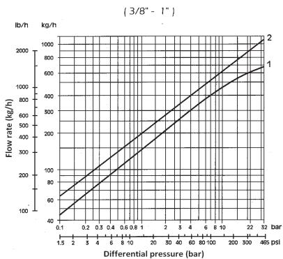
Curve 1: discharge 10 °C below the saturated curve Curve 2: discharge 20 °C below the saturated curve
