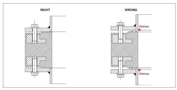
When mounting the pipe connector, make sure the pipe connector / flange surface is cleared from welding debrises, oil, paint, etc. Particular case shall be taken to ensure the storage area is kept cleaned.
