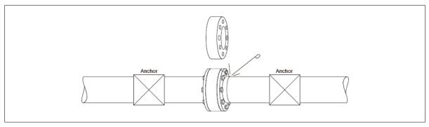
The pipe connector is made of rubber, heat shall be strictly eliminated during installation. Particular care shall be taken against sparks from welding, grinding, etc near the spot of connector installation.
