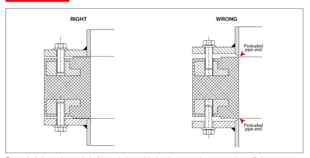
Protruded sharp pipe end shall be strictly avoided as it causes damage on / cut off pipe connector contact surface.
