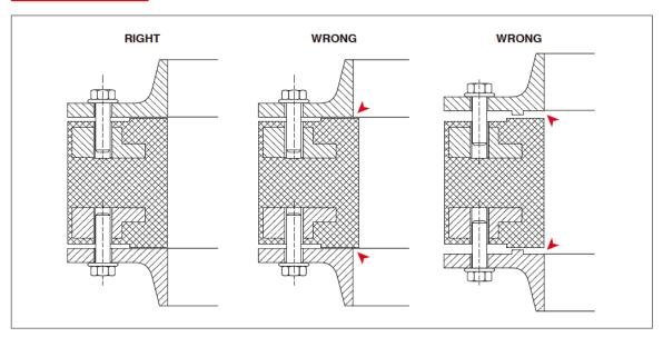
The use of the right mating flanges is important when fix the pipe connector. The flanges must cover the whole of the sealing surface of the pipe connectors.
