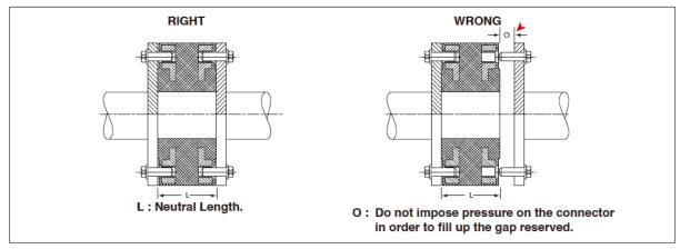
Mount pipe connectors shall be effected with the existent state maintained as it is. Particular care shall be taken to ensure the pipe connector must be free of tensile, shear, torsion or bending stresses during installation.
