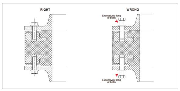
Use the correct length of bolts as excessively long of bolts will press the rubber body away from the flanges.
