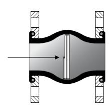
AISI 316 Ti vacuum ring (vacuum up to 1 bar) Ref.9815050 to 9815300
