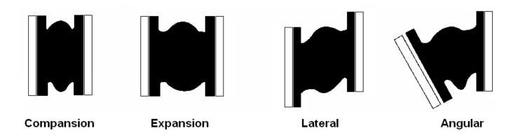
Maximum movements can't be applied simultaneously. For example, with an expansion of 15mm, the maximum lateral movement will be 8 mm :
