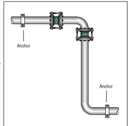
Arrangement with lateral expansion joints
