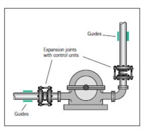
Pressure-restrained expansion joint on pump (with tie bar). Absorb vibrations and thus relieve pressure on the machine housing.
