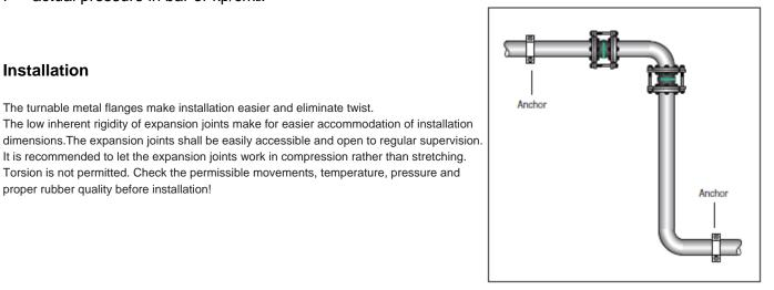
Arrangement with lateral expansion joints
