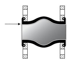
Inner liner PTFE (movements allowed by the expansion joints are then reduced by 50 % and pressure max is 6 bars)
