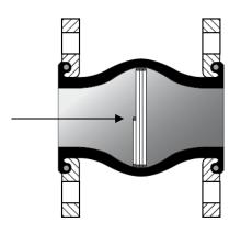
AISI 316 Ti vacuum ring (vacuum up to 1 bar) Ref.9815050 to 9815300
